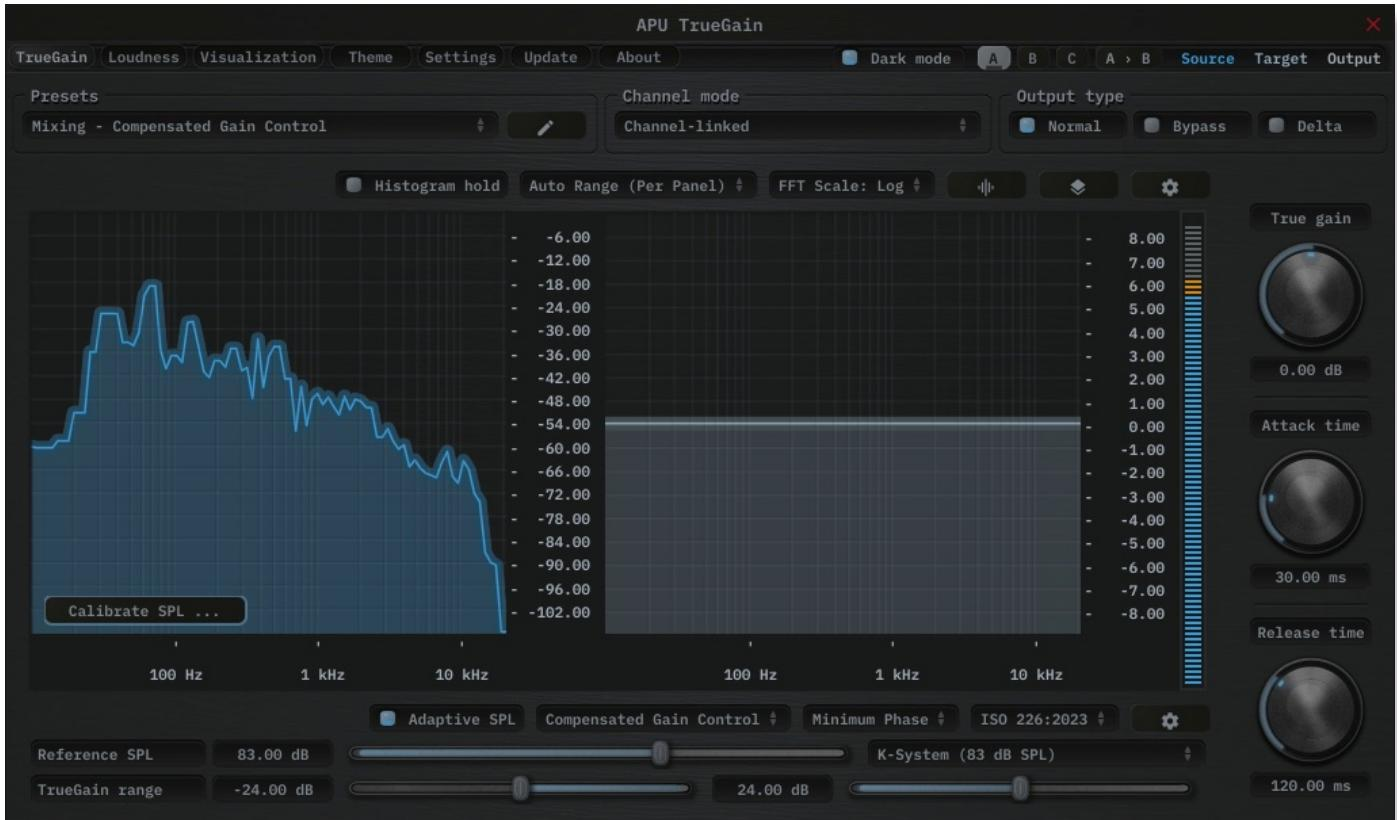
The TrueGain tab contains configuration and visualization for equal-loudness based gain compensation. This section details each of the individual parameters and components.
