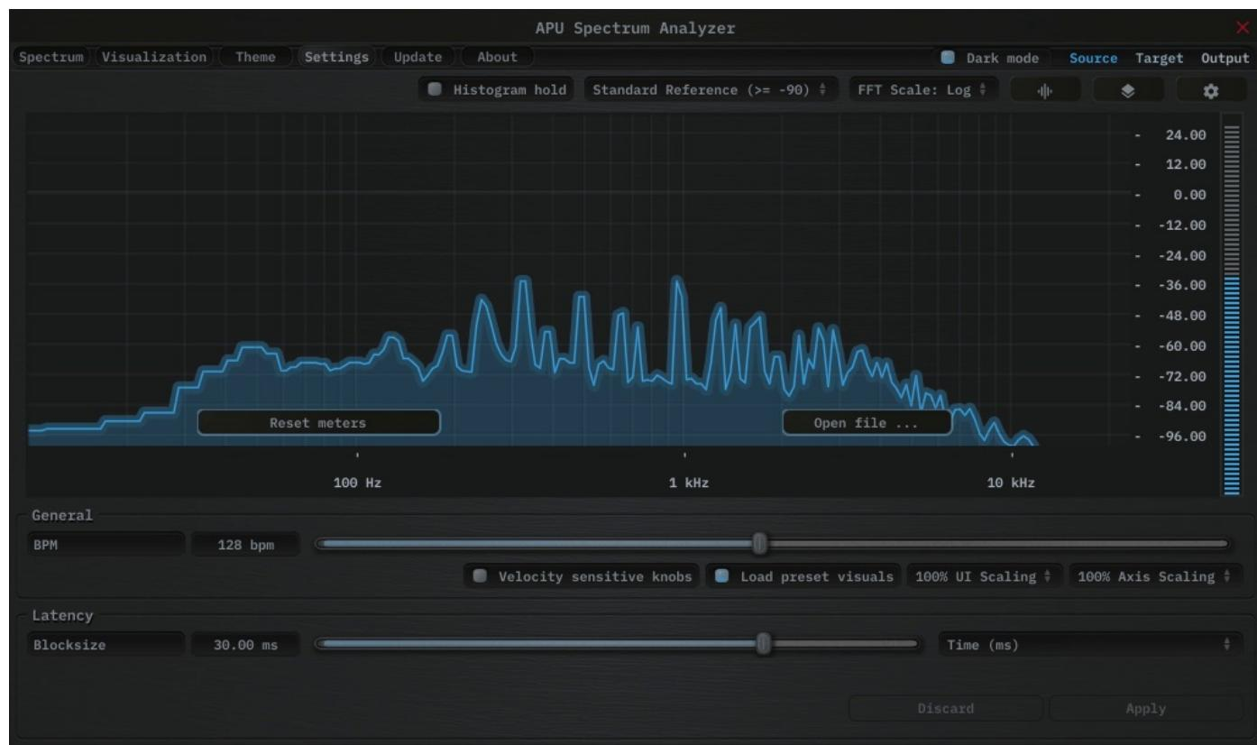
The settings tab contains various additional parameters. These parameters are broken down between General and Latency parameters. Since Latency parameters impact [delay compensation](#), changes to these parameters are deferred until you click the Apply button. It is generally not advisable to automate the parameters in the Latency section.
