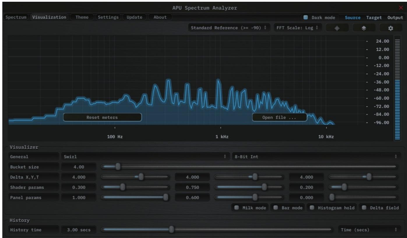
The visualization tab contains parameters related to real-time configuration of Spectrum Analyzer's visualizations. This section describes these various settings.
