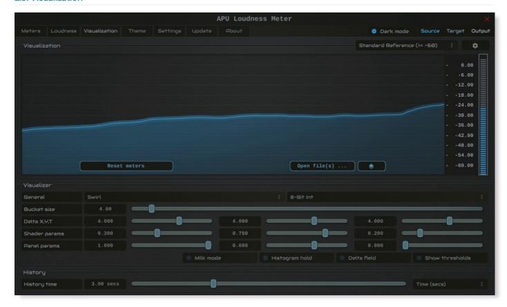
The visualization tab contains parameters related to real-time configuration of the meter's visualizations. This section describes these various settings.
