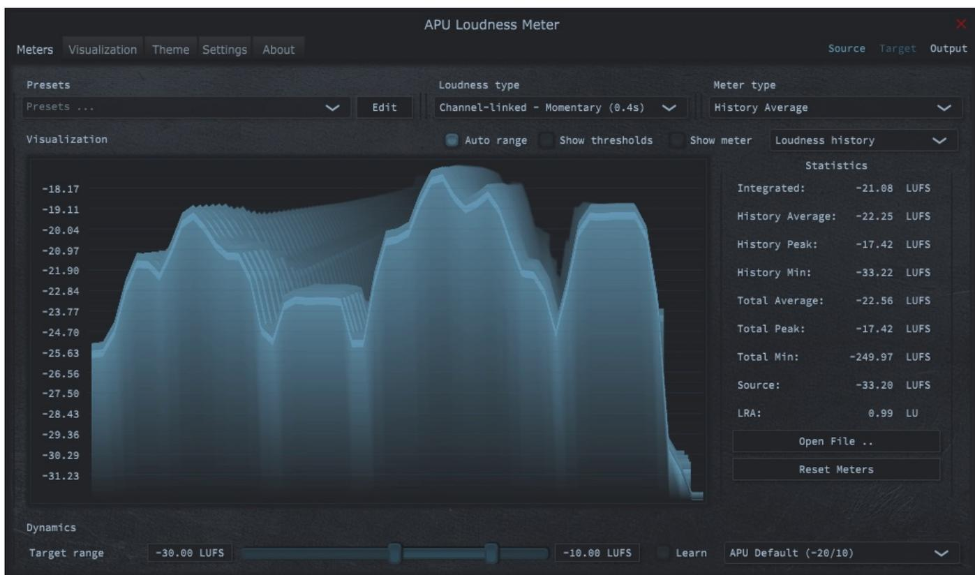
The meters tab contains configuration, visualization, and statistics for loudness analysis. This section details each of the individual parameters and components.
