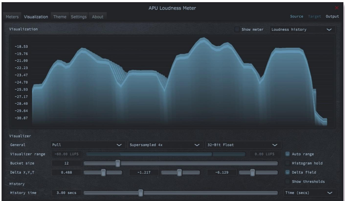
The visualization tab contains parameters related to real-time configuration of the meter's visualizations. This section describes these various settings.
