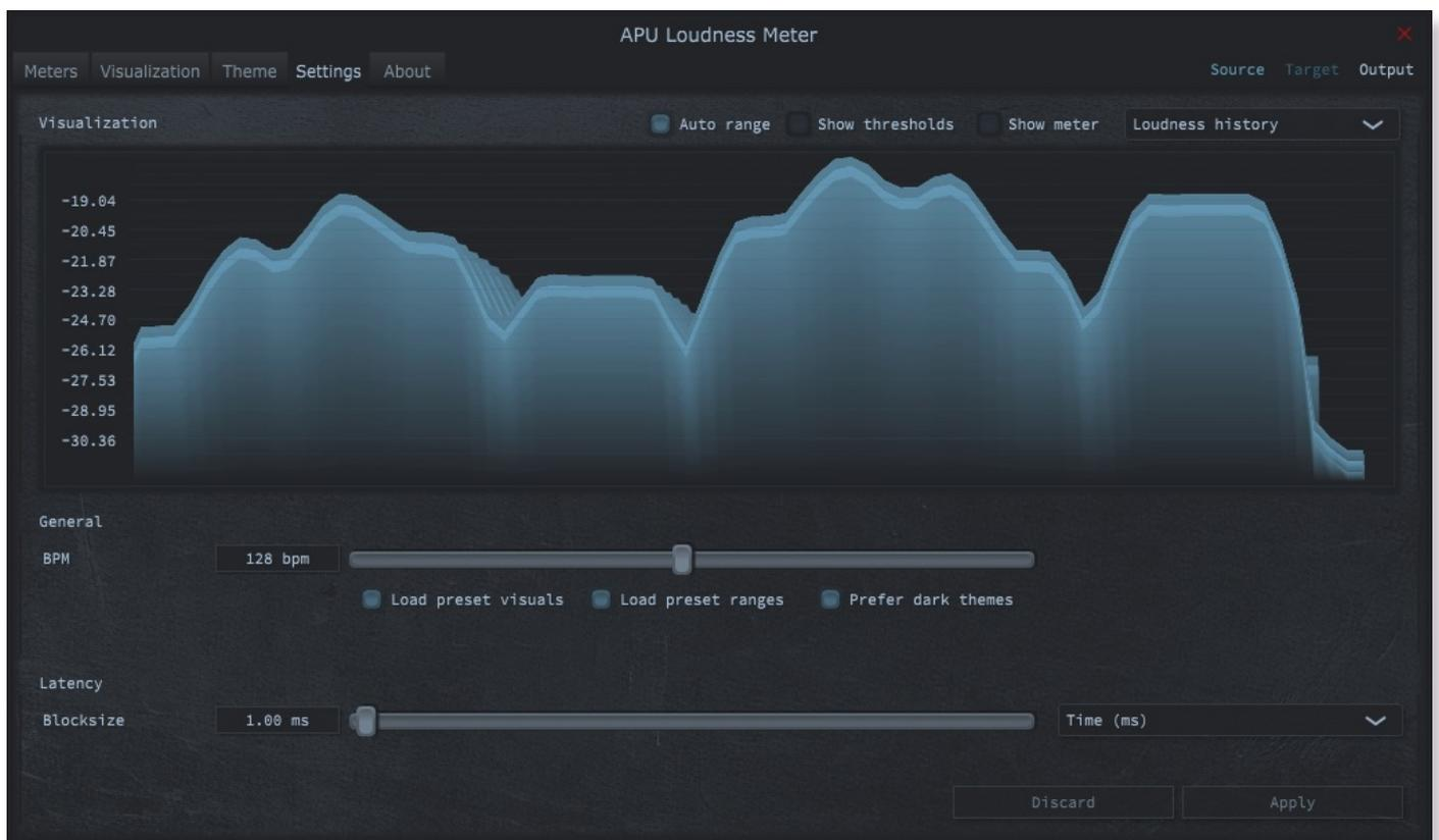
The settings tab contains various additional parameters. These parameters are broken down between General and Latency parameters. Since Latency parameters impact [delay compensation](#), changes to these parameters are deferred until you click the Apply button. It is generally not advisable to automate the parameters in the Latency section.
