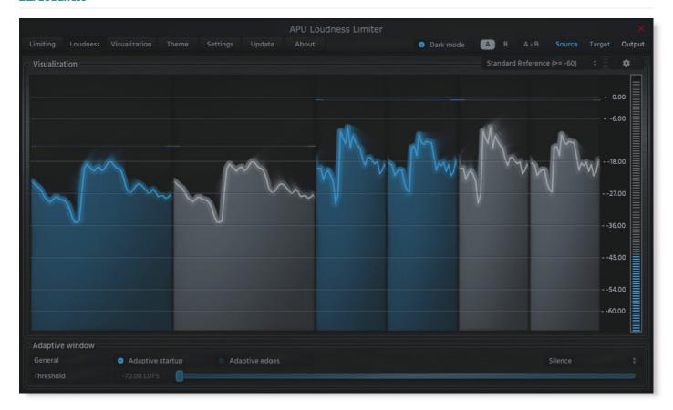
The loudness tab contains parameters relating to loudness measurements. You can configure adaptive window behavior here, which can be used to reduce transient artifacts during compression.
