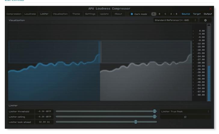
The limiter tab contains parameters relating to the built-in limiter. The limiter scans the <u>limiter lookahead</u> region of blocks for peak or true peak loudness values over the <u>limiter ceiling</u>. When these peaks are encountered, the current gain reduction trajectory is adjusted to accommodate the peak.
