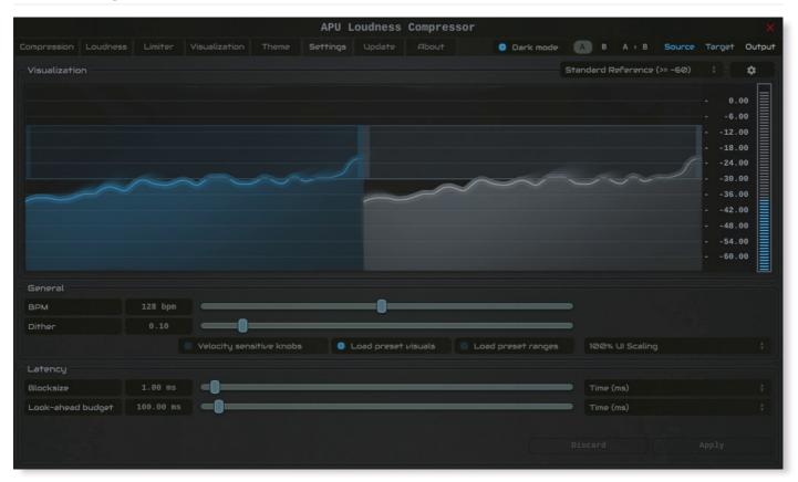
The settings tab contains various additional parameters. These parameters are broken down between General and Latency parameters. Since Latency parameters impact <u>delay compensation</u>, changes to these parameters are deferred until you click the Apply button. It is generally not advisable to automate the parameters in the Latency section.
