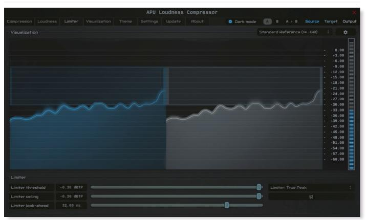
The limiter tab contains parameters relating to the built-in limiter. The limiter scans the <u>limiter</u> <u>lookahead</u> region of blocks for peak or true peak loudness values over the <u>limiter ceiling</u>. When these peaks are encountered, the current gain reduction trajectory is adjusted to accomodate the peak.
