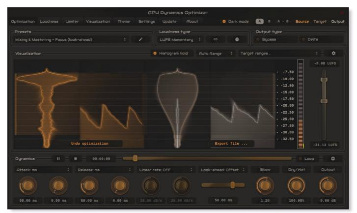
The optimizer's presets combo-box contains a collection of basic presets, one for each combination of <u>loudness type</u> and latency configuration. The low-latency presets introduce minimal delay, while the lookahead presets introduce more delay in exchange for the ability to preemptively respond to the source signal.
