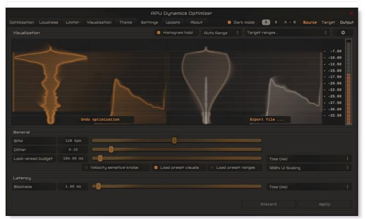
The settings tab contains various additional parameters. These parameters are broken down between General and Latency parameters. Since Latency parameters impact analysis, changes to these parameters are deferred until you click the Apply button, and will require the current file to be closed.
