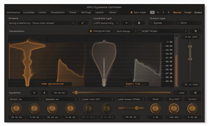
The optimization tab leads you through the optimization process. First, you can open an audio file for analysis. You can either use the file open button to browse for a file, or you can drag and drop a file onto the window. From that point, you'll be able to select a range of the audio to optimize.
