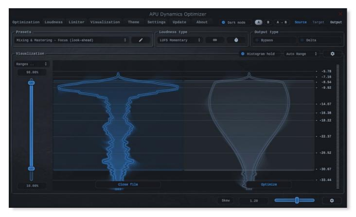
Once you have selected a range, you can press the right arrow button to perform the optimization. After optimization is complete, you can use the playback controls to listen to the results. From here you can make adjustments to <a href="attack/release">attack/release</a> and other parameters. Once you are happy with the results, press the downward arrow button to render to 32-bit float wav file.
