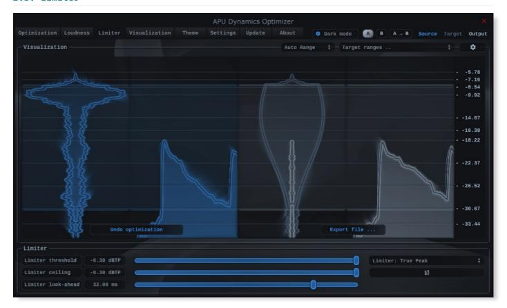
The limiter tab contains parameters relating to the built-in limiter. The limiter scans the <u>limiter</u> <u>lookahead</u> region of blocks for peak or true peak loudness values over the <u>limiter ceiling</u>. When these peaks are encountered, the current gain reduction trajectory is adjusted to accommodate the peak.
